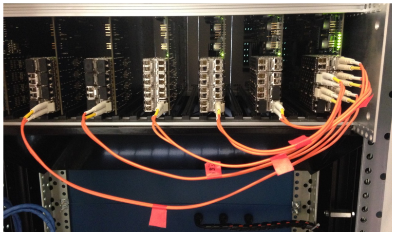
Figure 1. Card-to-card connection example for all-PB5 rack
