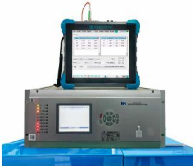
PNS330i test digital protective relay (SMV + GOOSE)
