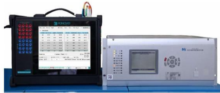
L336EXi test full digital protective relay (SMV sending + GOOSE subscription)
