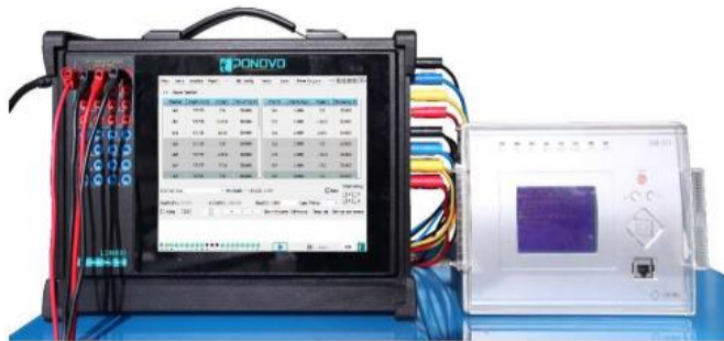
L336EXi test traditional protective relay (analog output + binary input)
