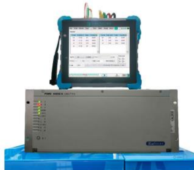
PNS330i send analog to MU, MU feedback SMV
