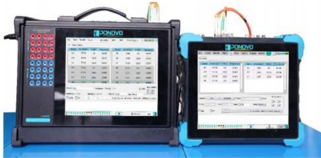
L336EXi receive SMV and GOOSE from PNS330i (SMV receive + GOOSE subscription)
