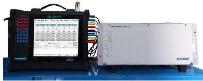
L336EXi send analog to MU, MU feedback SMV (Analog output+ SMV receive)
